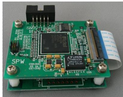
Fig. 4: Prototype module of SpaceWire thermal interface node
