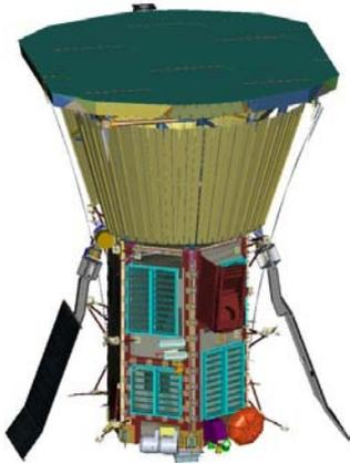
Since the solar arrays are necessarily exposed to a higher than typical solar flux during encounter, an active cooling system is required. This cooling system consists of water cooled solar array substrates and a mechanical pump loop which transfers heat from the solar arrays to radiators located under the TPS. Active cooling requires mass and consumes power, and thus the arrays must be minimally exposed, which in turn limits power.
