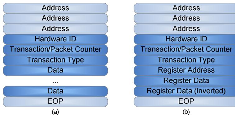
**Figure 5 Packet definitions for Process Request/Reply and Stream (a), and for Register Read/Write Request/Reply (b)**
