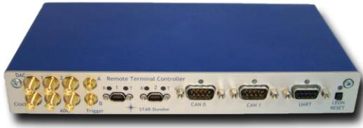
Figure 2 - SpaceWire RTC Development Unit front view
