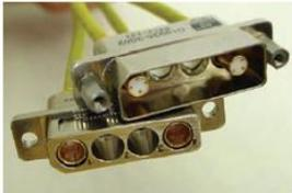
The suggested connectors are quadraaxial cable connectors containing two 100 Ohms impedance matched pairs per insert with the shield carried through the insert, which provides a continuous EMI shield for all signals.
