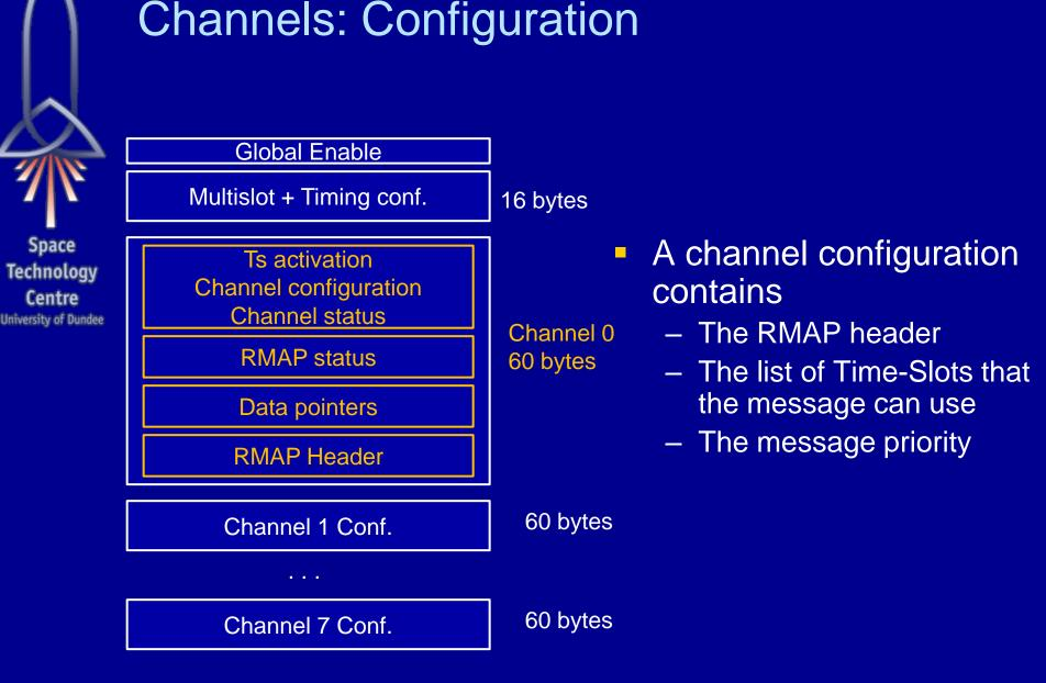
All configuration can be programmed with a single RMAP packet
